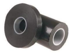
WRAP tapes are self-amalgamating modified polyisobutylene tapes, designed to stretch and stick to itself, forming a very strong and waterproof bond without leaving sticky stains on boat fittings.
