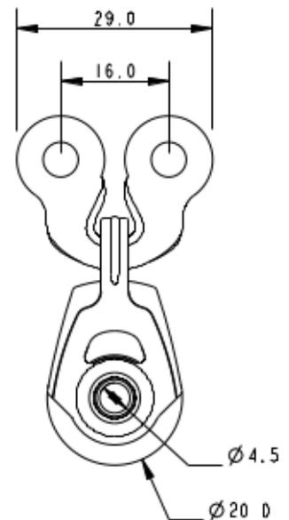
**Details:** The A2020P-4036 is a plain bearing block attached to an A4036 lacing eye. The A2020P is made using 100% recycled plastics and the well-known Allen Ultra-Strap. Ideal for elastic take up systems or any other application where dynamic performance is not vital. This block looks very similar to the 20mm dynamic version. To differentiate we have changed the sheave colour to grey.
