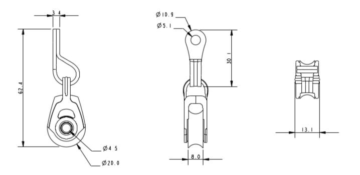
Details: The A2020P-4035 is a plain bearing block attached to an A4035 P-Clip. The A2020P is made using 100% recycled plastics and the well-known Allen Ultra-Strap. Ideal for elastic take up systems or any other application where dynamic performance is not vital. This block looks very similar to the 20mm dynamic version. To differentiate we have changed the sheave colour to grey.
