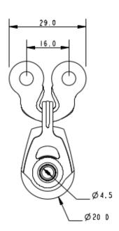
Details: The A2020P-4036 is a plain bearing block attached to an A4036 lacing eye. The A2020P is made using 100% recycled plastics and the well-known Allen Ultra-Strap. Ideal for elastic take up systems or any other application where dynamic performance is not vital. This block looks very similar to the 20mm dynamic version. To differentiate we have changed the sheave colour to grey.
