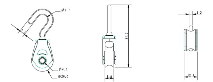
Details: The A2020PSHK is a plain bearing block with a swivel hook attachment. The A2020PSHK is made using 100% recycled plastics and the well-known Allen Ultra-Strap. Ideal for elastic take up systems or any other application where dynamic performance is not vital. This block looks very similar to the 20mm dynamic version. To differentiate we have changed the sheave colour to grey.
