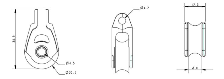
Details: The A2021P is a plain bearing block with multi functional head, ideal for use with shackles or clevis pins. The A2021P is made using 100% recycled plastics and the well-known Allen Ultra-Strap. Ideal for use in elastic take up systems or applications where dynamic performance is not vital. This block looks very similar to the 20mm dynamic version. To differentiate we have changed the sheave colour to grey.
