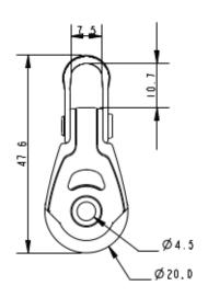
Details: The A2022P is a plain bearing version of our A2022 dynamic double block. The A2022P is made using 100% recycled plastics and the well-known Allen Ultra-Strap. Ideal for use in elastic take up systems or applications where dynamic performance is not vital. This block looks very similar to the 20mm dynamic version. To differentiate we have changed the sheave colour to grey.
