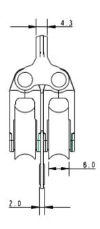
Details: The A2023P is a plain bearing version of our A2023 dynamic double with becket block. The A2023P is made using 100% recycled plastics and the well-known Allen Ultra-Strap. Also featuring a rope friendly becket the A2023P is Ideal for elastic take up systems. This block looks very similar to the 20mm dynamic version. To differentiate we have changed the sheave colour to grey.
