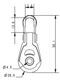
Details: The A2024P is a plain bearing version of our A2024 dynamic cheek block. The A2024P is made using 100% recycled plastics and the well-known Allen Ultra-Strap. Ideal for elastic take up systems. This block looks very similar to the 20mm dynamic version. To differentiate we have changed the sheave colour to grey.
