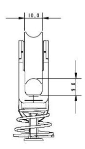
Details: The A2030PLZ is created using a standard A2030P plain bearing block attached to a A4073 lacing eye with a A4034 conical spring to hold the block upright. The A2030P is manufactured using 100% recycled plastics and our patented Ultra-Strap. Ideal for applications which do not require a dynamic performance. This block looks very similar to the 30mm dynamic version. To differentiate we have changed the sheave colour to grey.
