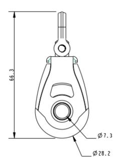
Details: The A2030PSC plain bearing swivel block is manufactured using 100% recycled plastics and our recognisable stainless steel side cheeks. The swivel on the head of the block allows the block to rotate to which ever angle is best for the sheet. Ideal for elastic take up systems. This block looks very similar to the 30mm dynamic version. To differentiate we have changed the sheave colour to grey.
