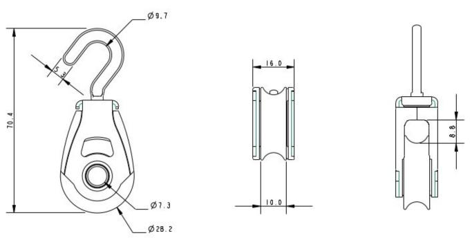
Details: The A2030PSHK is a plain bearing block with a swivelling hook attachment. The A2030PSHK is made using 100% recycled plastics and reinforced with our recognisable stainless steel side cheeks. Ideal for elastic take up systems. This block looks very similar to the 30mm dynamic version. To differentiate we have changed the sheave colour to grey.
