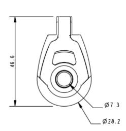
Details: The A2031P is a plain bearing version of our A2031 dynamic block. The A2031P is made using 100% recycled plastics and the well-known Allen Ultra-Strap. This block also features the multi function head, allowing a better fit for small shackles or clevis pins. This block looks very similar to the 30mm dynamic version. To differentiate we have changed the sheave colour to grey.
