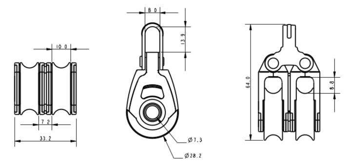
Details: The A2032P is a plain bearing version of our A2032 dynamic cheek block. The A2032P is made using 100% recycled plastics and the well-known Allen Ultra-Strap. Ideal for elastic take up systems. This block looks very similar to the 30mm dynamic version. To differentiate we have changed the sheave colour to grey.
