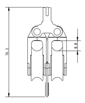
Details: The A2033P is a plain bearing double block with additional becket. The A2034P is made using 100% recycled plastics and the well-known Allen Ultra-Strap. Also featuring a rope friendly becket the A2033P is Ideal for elastic take up systems. This block looks very similar to the 30mm dynamic version. To differentiate we have changed the sheave colour to grey.
