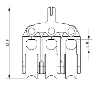
Details: The A2034P is a plain bearing triple block. The A2034P is made using 100% recycled plastics and the well-known Allen Ultra-Strap. Ideal for elastic take up systems. This block looks very similar to the 30mm dynamic version. To differentiate we have changed the sheave colour to grey.
