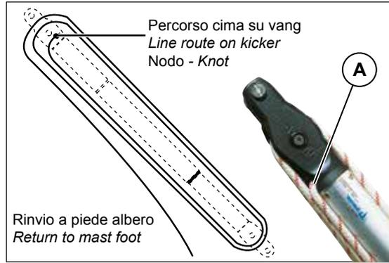
Insert line in hole (A), make a knot on the extremity and follow the route presented in the drawing.
