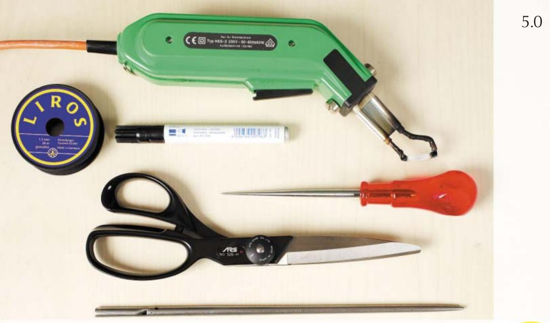
Tools needed for an endless splice.
