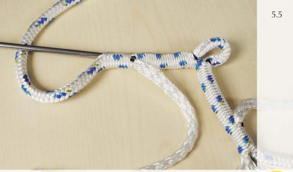
Now insert the other core at the other 15 cm mark and push it through to the 30 cm mark where the core came out. If possible exit 20 cm past the 30 cm mark.
