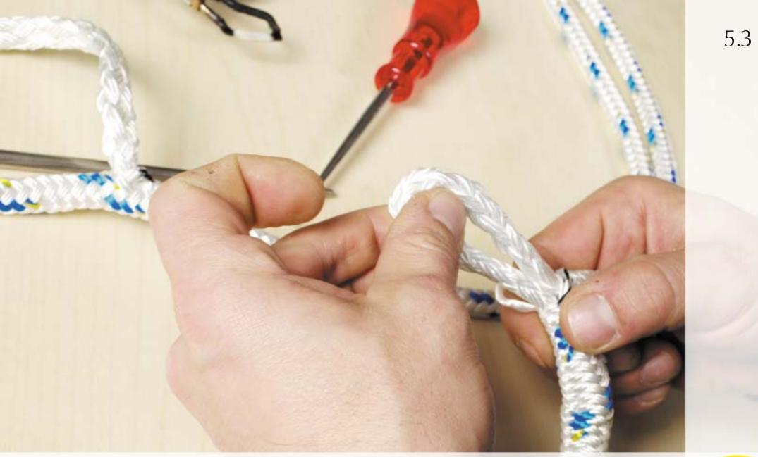
Photo showing the core pulled out.
