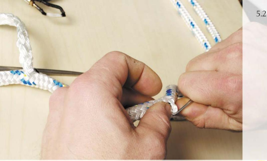
Pull the core out of the cover at the two 30 cm markings.
