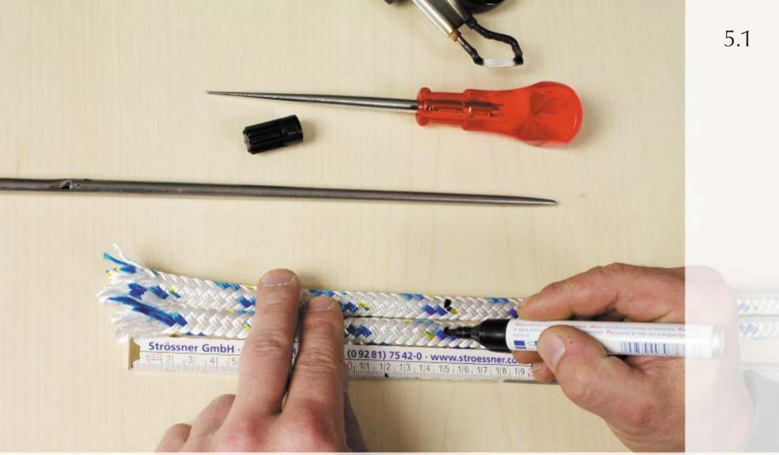
Mark both ends of the rope at a point 15 x 30 cm from each end of the rope to be spliced.
