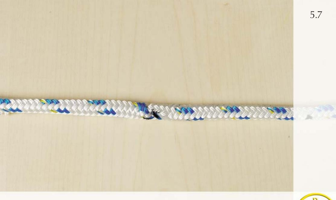
After "milking" the cover down completely cut off the rope ends that are protruding so the ends can be "milked" into the core.
