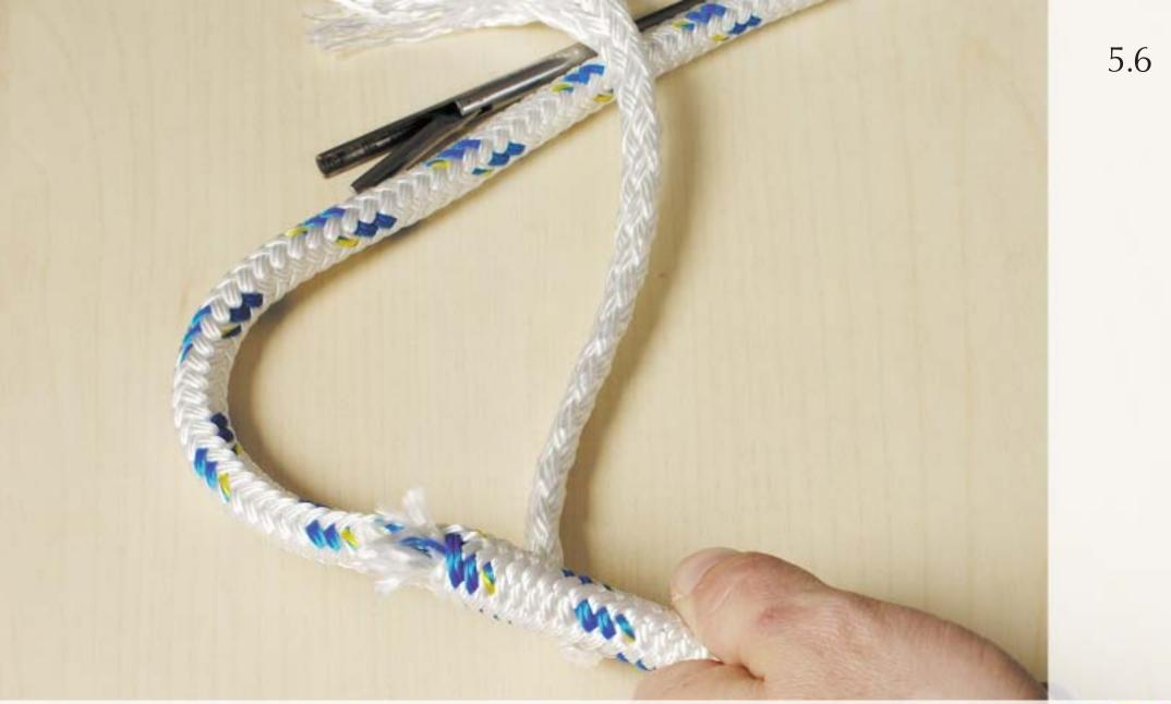
"Milk" the cover down over the core so that the cover on the inside and the other core finish flush with each other.
