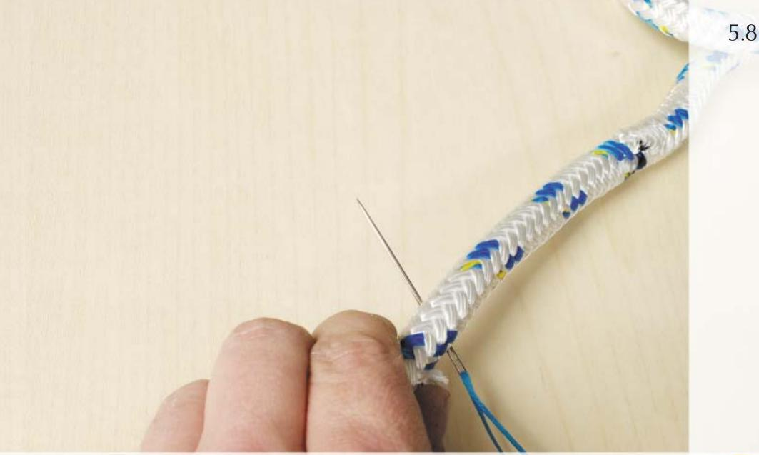
Sew through the splice on sides of the centre several times to prevent any movement of the core.
