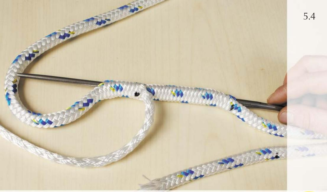
Feed the core into the fid and isert at the 15 cm mark and push it through towards the 30 cm mark where the core comes out. If possible make the exit 20 cm beyond the 30 cm.
