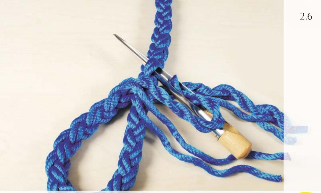
Insert the fid under two strands and feed the first pair through.
