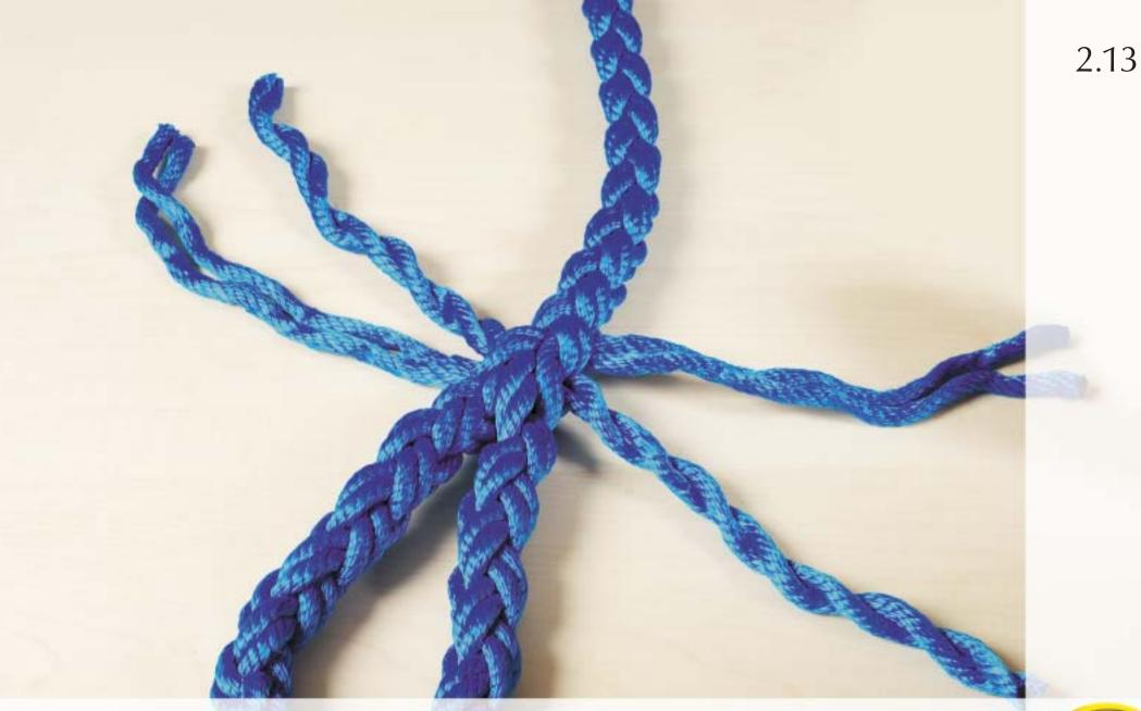
Make sure that the 4 pairs of strands are positioned exactly as per the picture.
