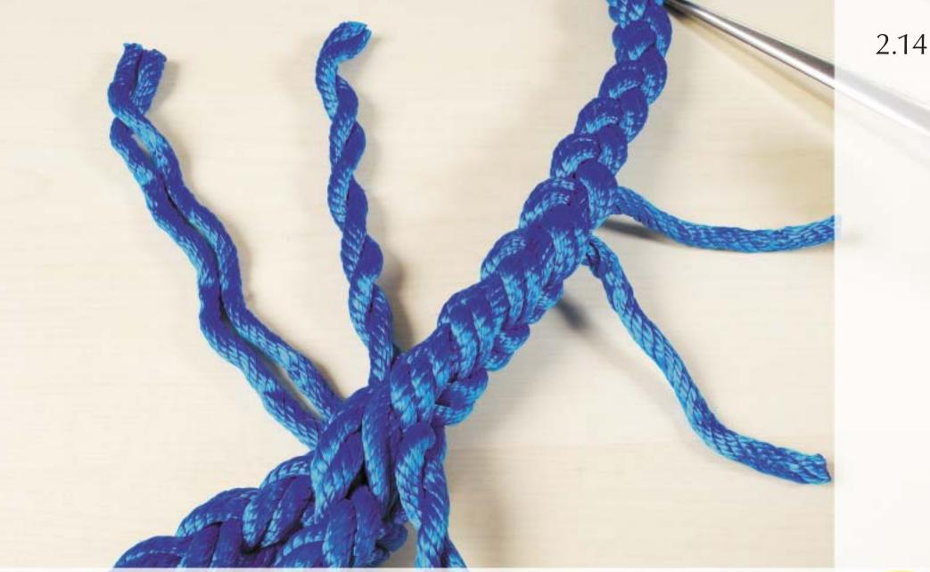
Make four further tucks down the rope with the first pair of strands. On the last tuck divide the pair into single strands so the splice becomes tapered.
