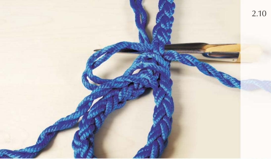
Using the fid insert the two strands from the left under the two strands.
