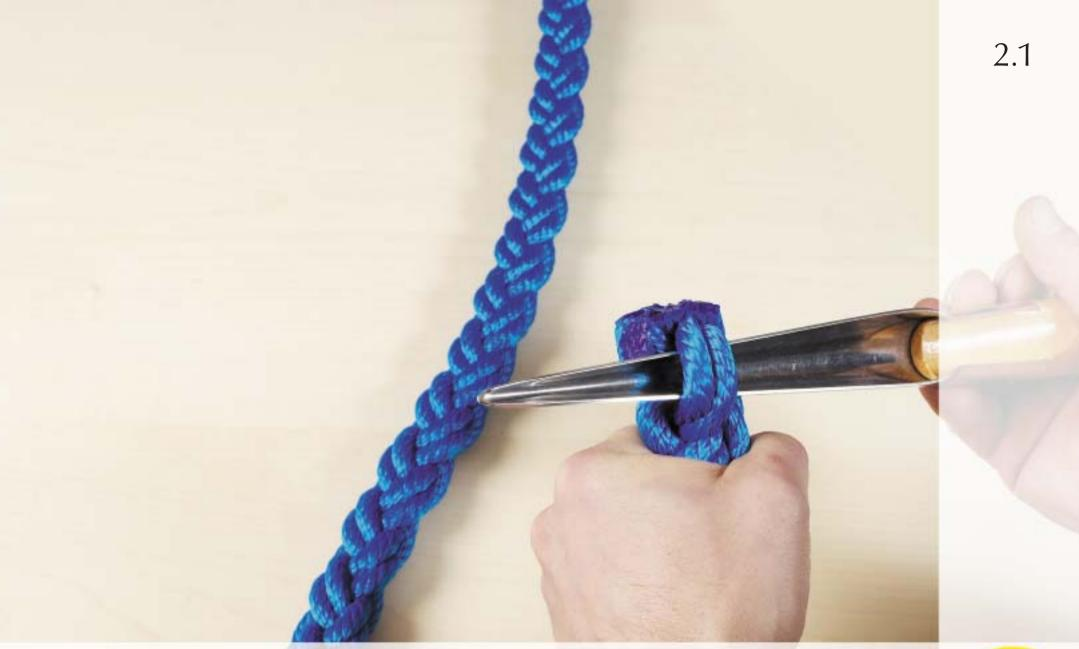
Open the rope by levering a pair of strands away from the main part of the rope. On completion the rope should divide into 4 pairs of 2.
