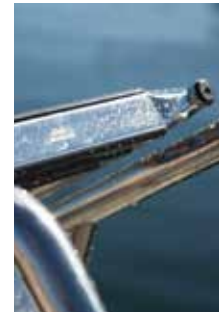
Pivoting handles For better stowing. (BUT45R)
