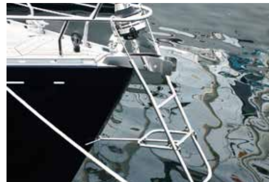
ST130AL is designed to fit a blunt stem, or a boat with stem anchor. The topmost step has been removed, and the upper edge is broadened, to make room for the anchor. The last step is foldable.
